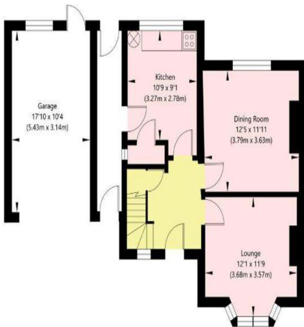
Ground Floor - (Excluding Garage) GROSS INTERNAL FLOOR AREA APPROX. 496 SQ FT / 46.12 SQ M
